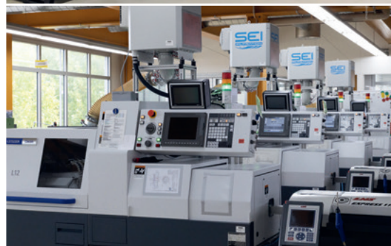
Dubois Dépraz operates an impressive fleet of machines. Shown here, Tornos Swiss Nano and Citizen 3 precision turning machines.
